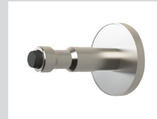
Single coat hook 65mm Stainless steel Contemporary stainless steel single coat hook with concealed fixings and precision made groove retained buffer. Load tested to 30kg. Ø50 x D65mm Code: MFC/HPL/CC CH65T SGL CH65SG
