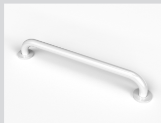
600mm straight grab rail Powder coated stainless steel Doc M and HBN compliant 600mm grab rail with concealed fixings. W600 x Ø35mm Code: White GRAB202 Blue GRAB205 Light Grey GRAB208 Dark Grey GRAB211
